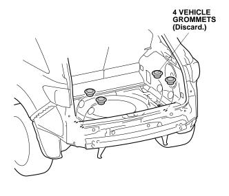
12. Insert the right and left trailer hitch plates through the grommet holes.
