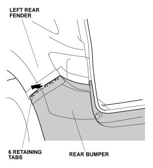
• Release one retaining tab on each side.
